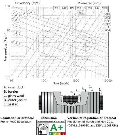
The SONODEC 25 GLX fulfills all the requirements and are classified as specified within EN 13180: Ventilation for buildings – Ductwork - Dimensions and mechanical requirements for flexible ducts.
